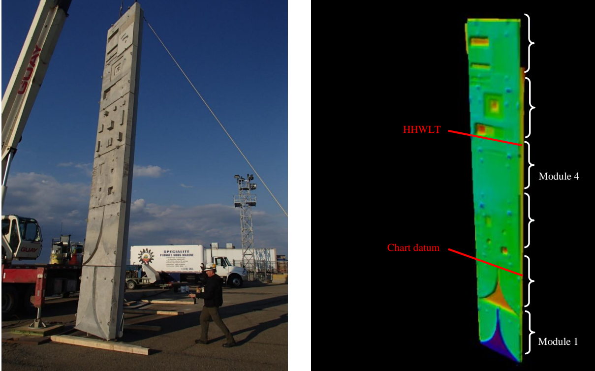
Figure 5 : Test bench just before deployment (left). VDTM of the test bench built from the HandyScan 3D reference dataset gridded at 2cm resolution.
