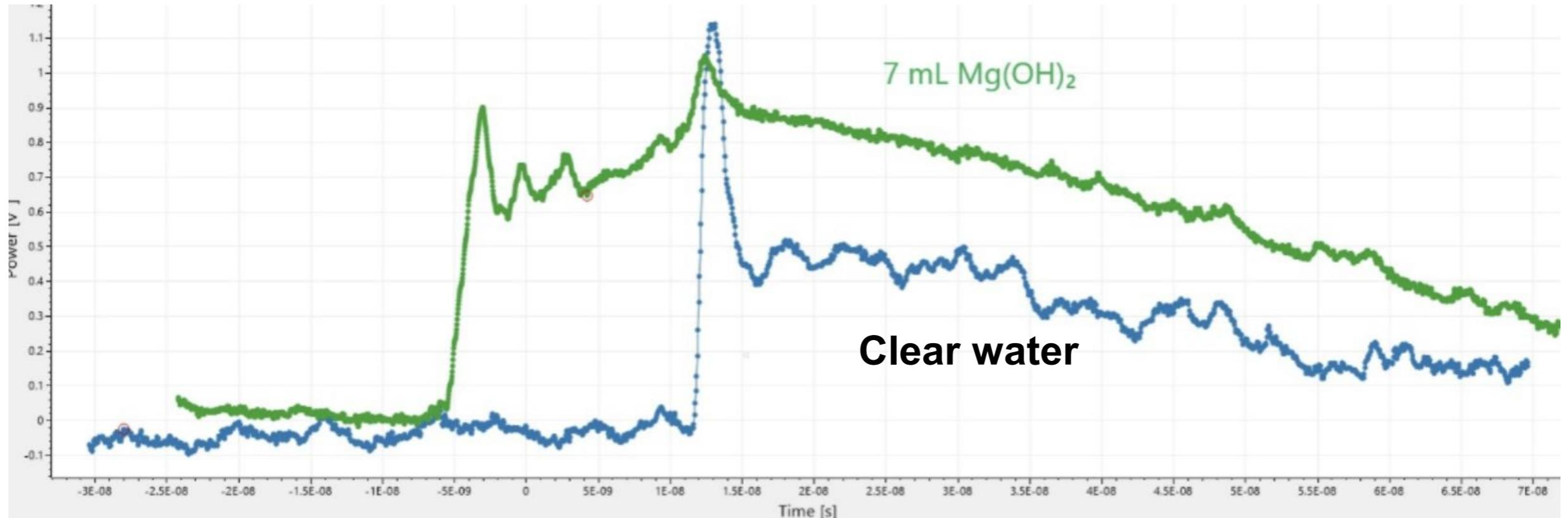
Full wave form comparison of clear water vs. mildly turbid water with sand target at 2 meter distance
